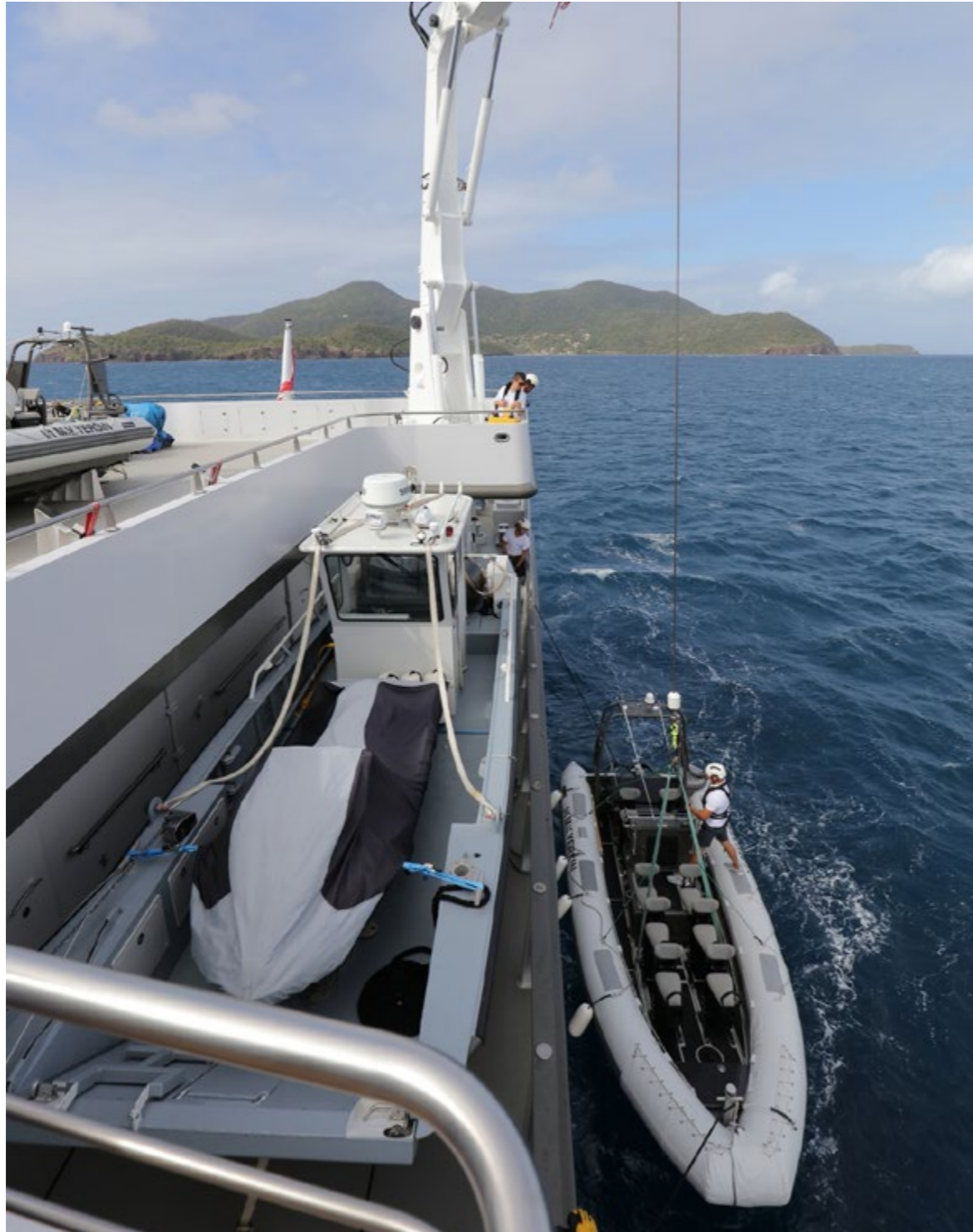
AFT CRANE HAULING 7.5M HURRICANE ZODIAC TENDER & MUNSON LANDING CRAFT STORAGE PORTSIDE
